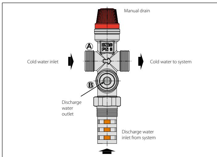
When the setting temperature is reached, the cold water inlet aperture (A) and the discharge aperture (B) are opened at the same time, until the temperature drops below the trigger value and the inlet and discharge apertures close simultaneously.
