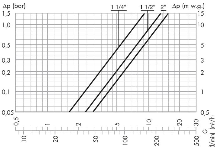
FLOW RATES recommended to ensure stable operation and accuracy of  $\pm 2^\circ\text{C}$  (balanced pressure Hot/Cold)
