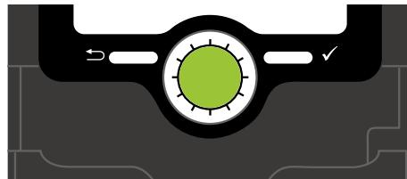
The control unit is controlled by means of 2 keys and 1 rotary switch (Lightwheel®) under the display:
