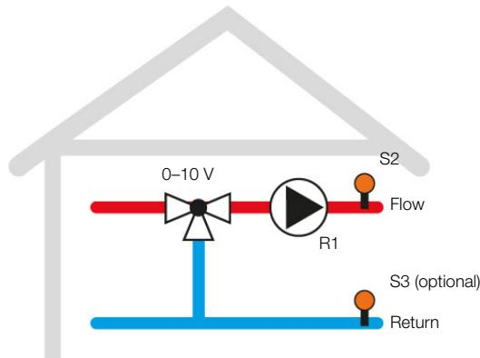
The controller monitors the room thermostat signal (RT). If the room thermostat requests energy, the pump (R1) and R4 are turned on to request heating. The temperature measured by probe S2 is monitored. The mixing valve is regulated to ensure that S2 reaches and maintains the set temperature **T Set**.
