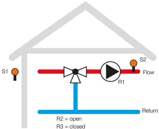
If the **Cooling** option is activated, the mixing valve is regulated to ensure that S2 reaches and maintains the cooling temperature **TCool**. As an option, contact S7 can be used for remote control of the heating / cooling function.
