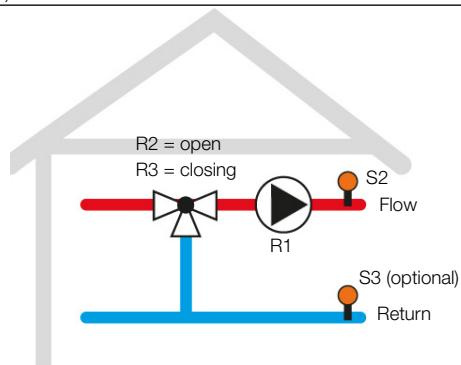
The controller monitors the room thermostat signal (RT). If the room thermostat requests energy, the pump (R1) and R4 are turned on to request heating. The temperature measured by probe S2 is monitored. The mixing valve is regulated to ensure that S2 reaches and maintains the set temperature **T Set**.
